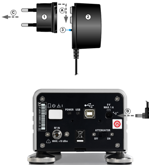
Fig. 4-5: Assembling the power supply adapter
